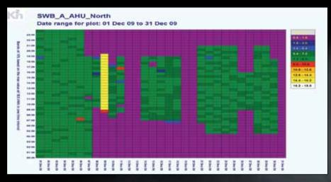
Sub-metering shows an AHU working outside office hours
